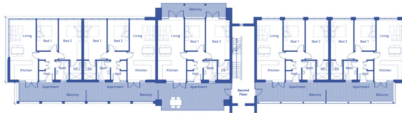
Typical Upper Level Apartment Plan (Level 3)
